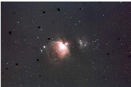
Figure 5: The use of flat frames. Light frames before flat correction having dust motes all across the image and vignetting at the edges have been used. Source
