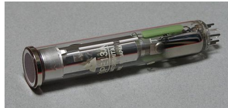
(b) vidicon(analog image sensor)
