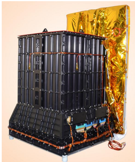
Figure 2.3: Fully assembled Cadmium Zinc Telluride Imager prior to its integration with the spacecraft.
